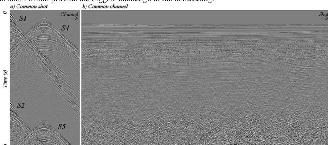
Figure 3 Raw recorded data, aligned on S1 firing time. a) Shot gather, b) Common channel gather.
