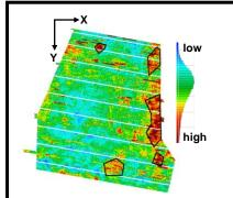
Figure 5: Map of the smallest similarity measurement (L2) value for each shot. Polygons around areas of poor similarity (large values) are used to select extra shots for the training.
