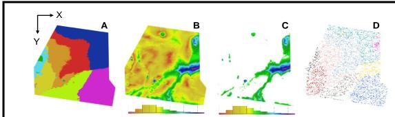
Figure 3 – A- Clusters obtained using the four horizons (8 clusters, each cluster is represented by one color). B- Distance to the centroid of the cluster. Blue indicates high distance to the centroid. C- Outliers from map B used to form new clusters. D- Positions of the training points (when selecting a percentage of data points per cluster), the colors corresponding to the 12 updated clusters.
