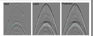
**Figure 1** – Shot point (Left) before deghosting, (Middle) after physics-based source and receiver deghosting (label) and (Right) after DNN prediction.
