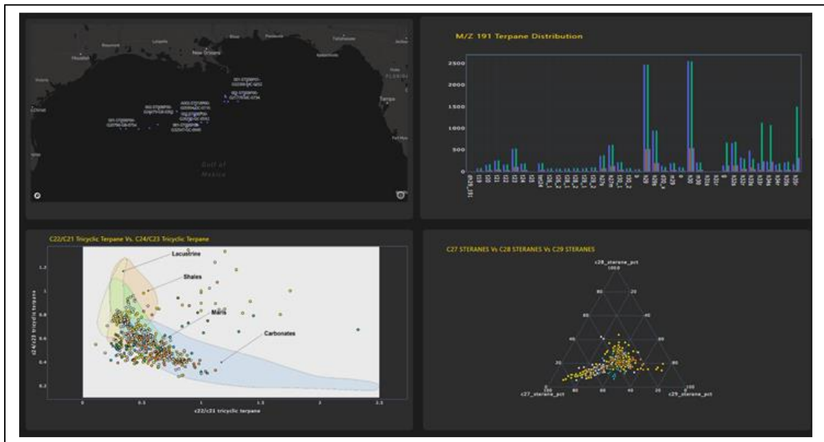
Figure 3 Data analytics on the saturate GC-MS dataset in the US GOM, including relative abundance diagrams, tricyclic cross plots and Sterane ternary diagrams.
