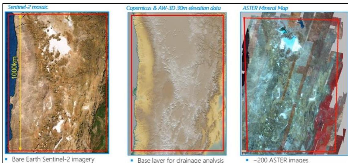
**Figure 1.** The use of optical Sentinel-2 imagery for the geological mapping, Copernicus and AW3D elevation data for the drainage analysis and ASTER for multi-spectral clay alteration mapping have enabled large-footprint paleosalars to be outlined.
